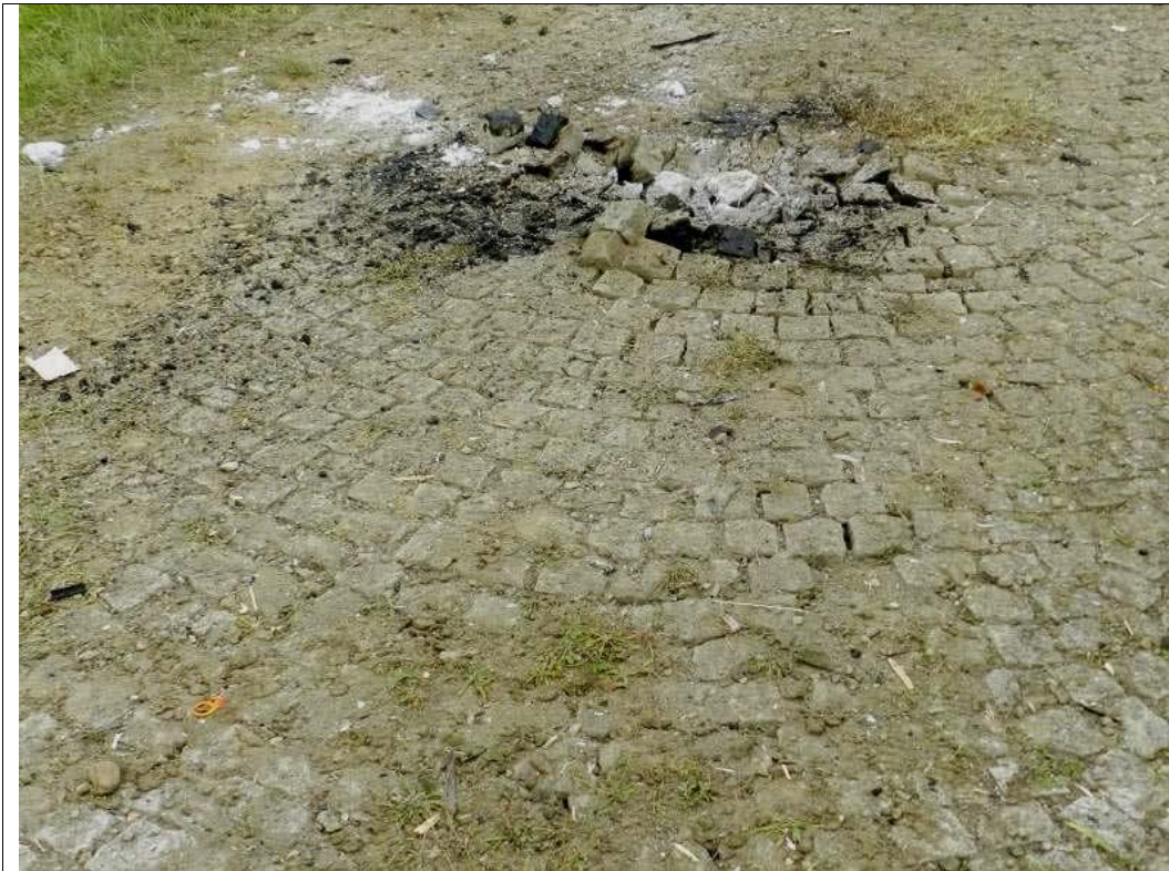
Figure 46 – The place of explosion of 2,5 kg of PEP 500 explosive placed under the bumper ( photograph DSCN0027 ).
