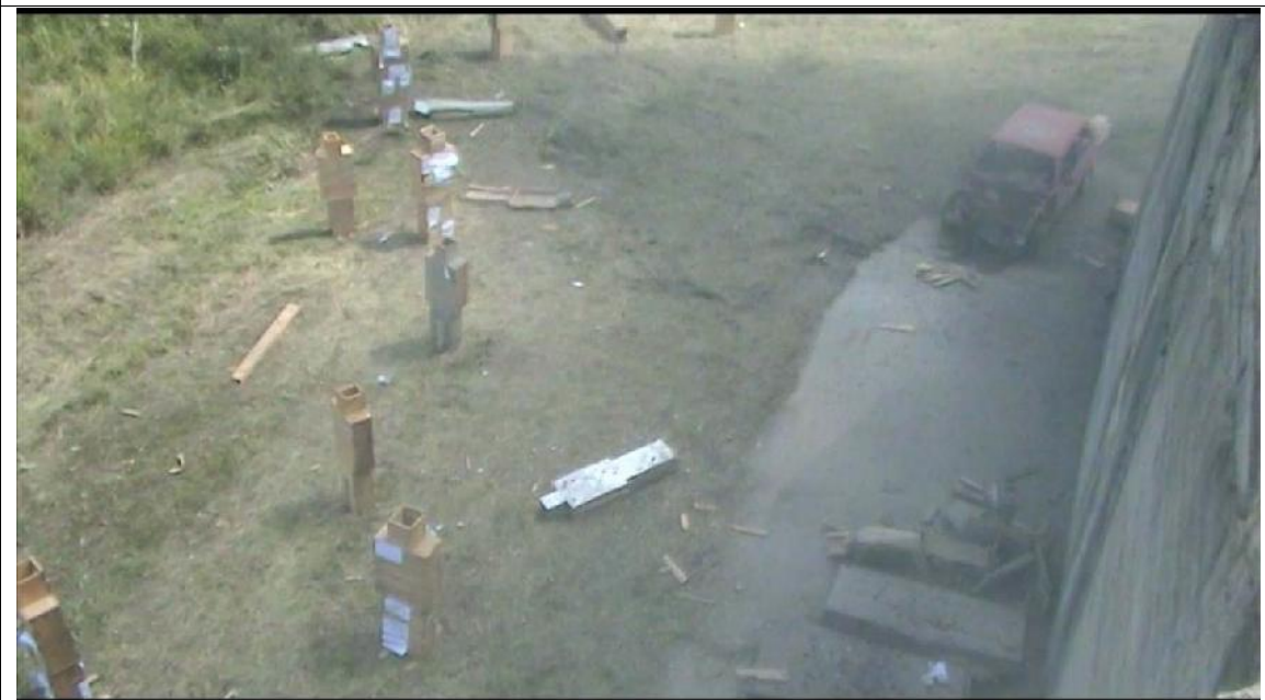
Figure 26 – The models and the car, before, during and after the explosion of 130 mm OF 482M projectile under the 43° descent angle
