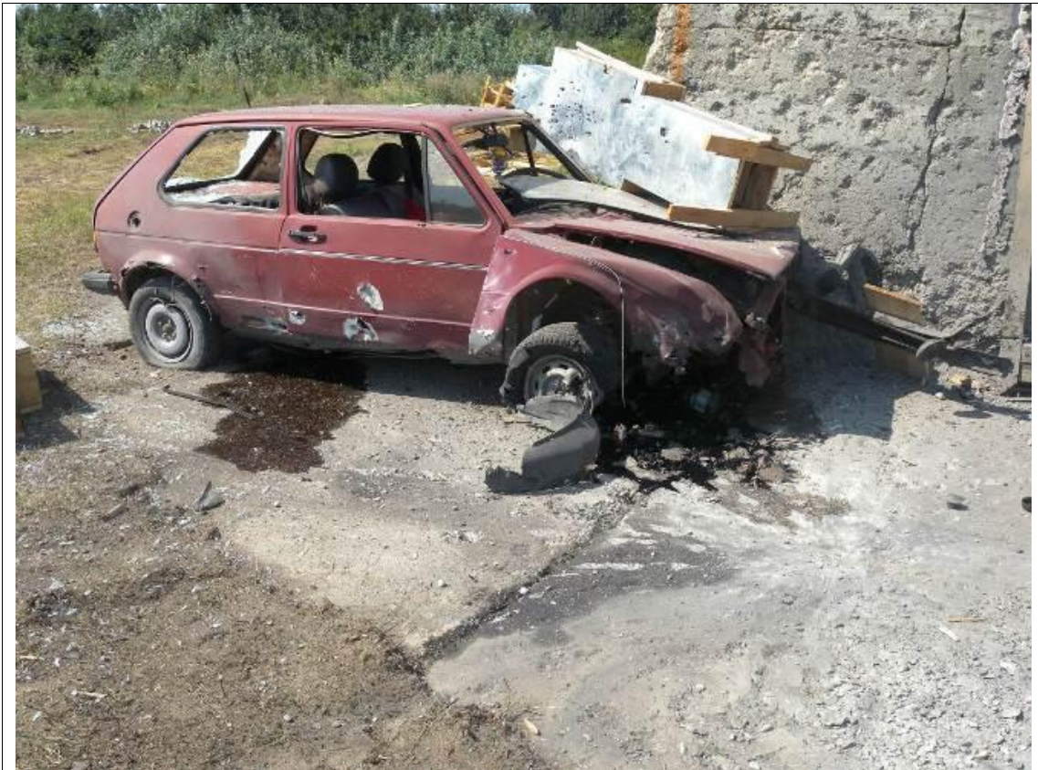
Figure 24 – The vehicle, type “Golf 1“ after the activation of 130 mm M79 projectile placed at the 62° angle to the horizon (photograph DSCN5605)
