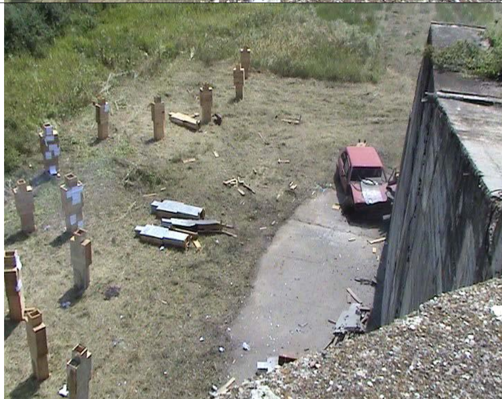
Figure 17 – The models and the car, before, during and after the explosion of 130 mm O 482M projectile at the angle of 62° angle
