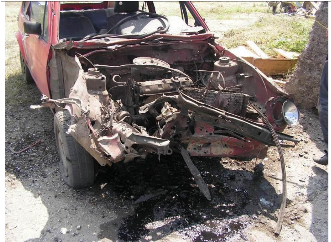
Figure 28 – The vehicle, type “Golf 1“ after the activation of 130 mm OF 482-M projectile placed under the 43° angle in relation to the horizon (photograph PICT0910)
