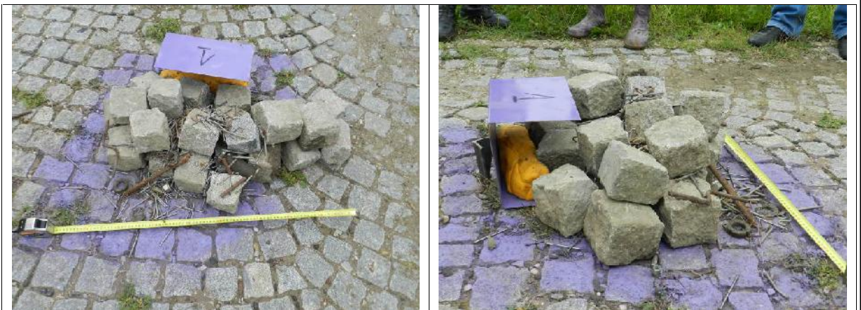
Figure 51 - 2,5 kg explosives immediately before activation 1- Tin deflector
