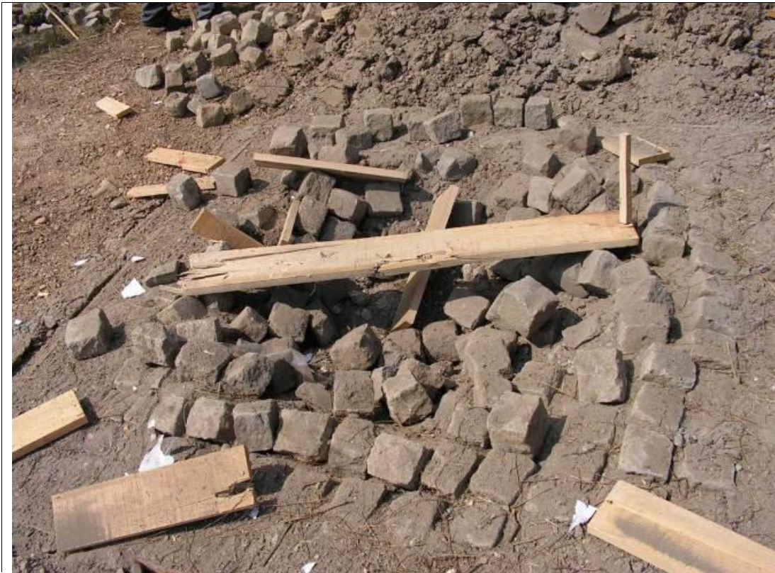
Figure 58 – The appearance of the place where 2,4 kg TNT was activated. The board over the crater was added later, for measurement of depth of the crater.
