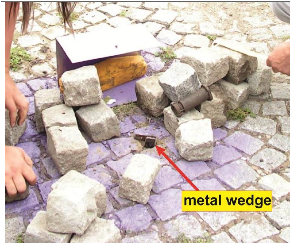
Photograph 52 – A metal wedge was nailed in front of the explosive at about 25cm
