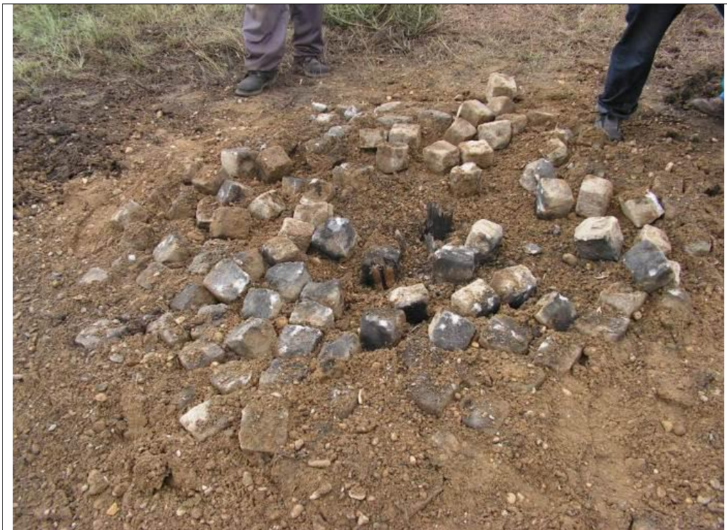
Figure 12 – The explosion place of the 130 mm M79 projectile, placed under the angle of 90°. (Photograph number PICT0486)
