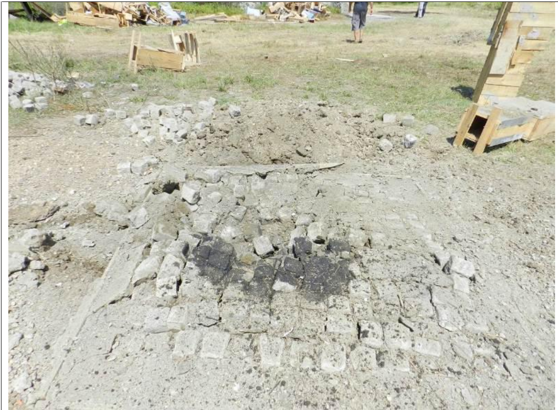
Figure 48 – The place of explosion of the 1 kg, PEP 500 explosive.
