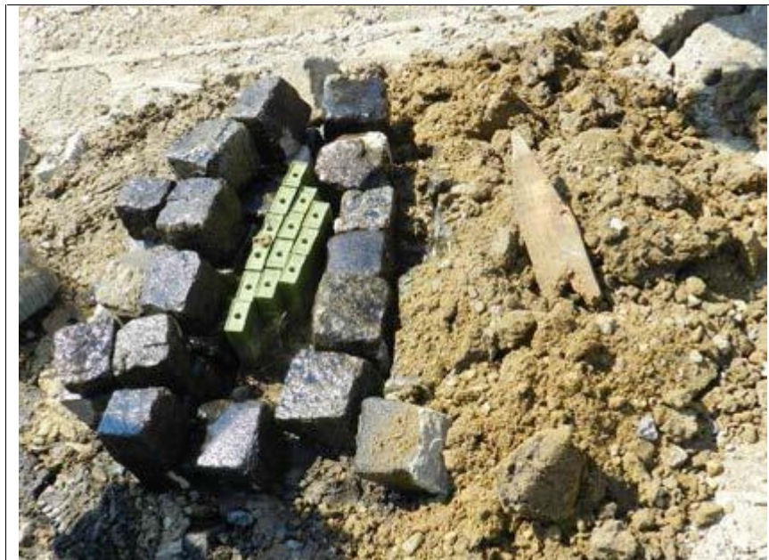
Figure 60 – The layout for 2,6kg of TNT on the granite cubes surface.
