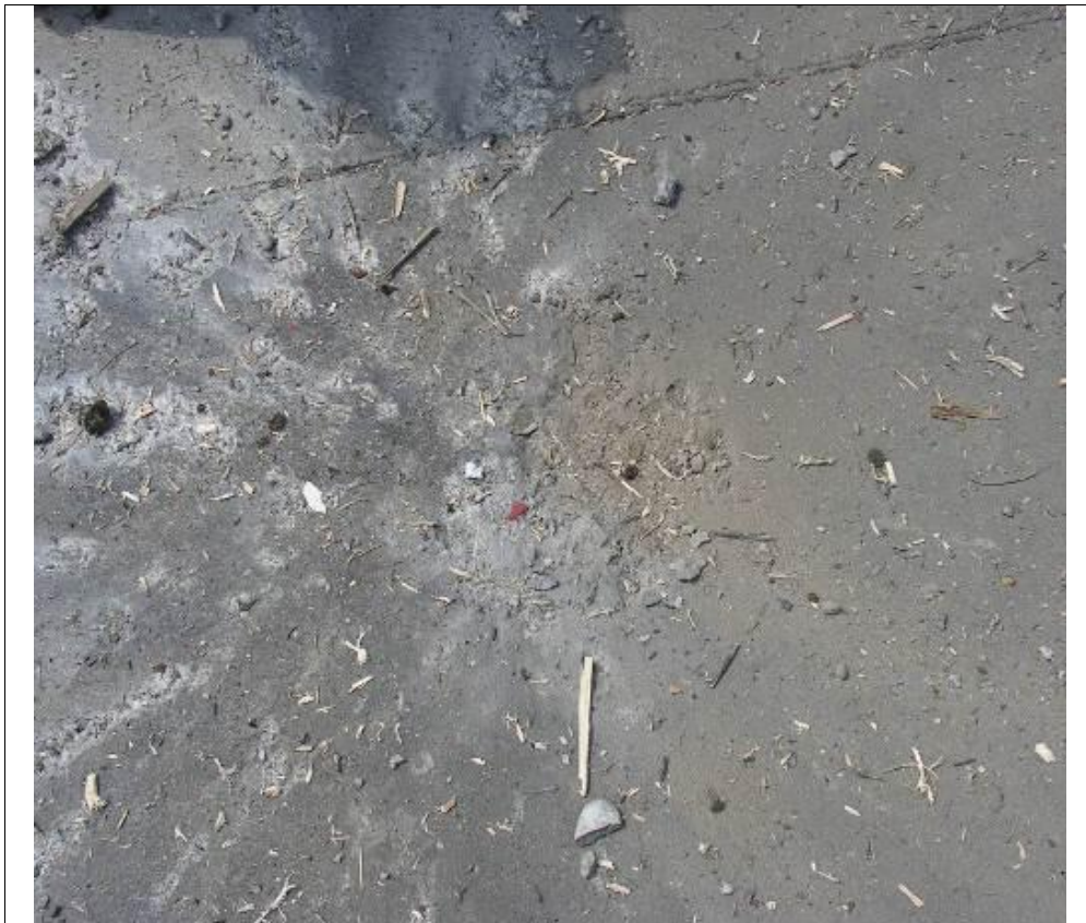
Figure 19 - The impression from the projectile pieces on concrete surface after the activation of 130 mm OF 482 M projectile placed at the 62° angle to the horizon (photograph PICT0748)
