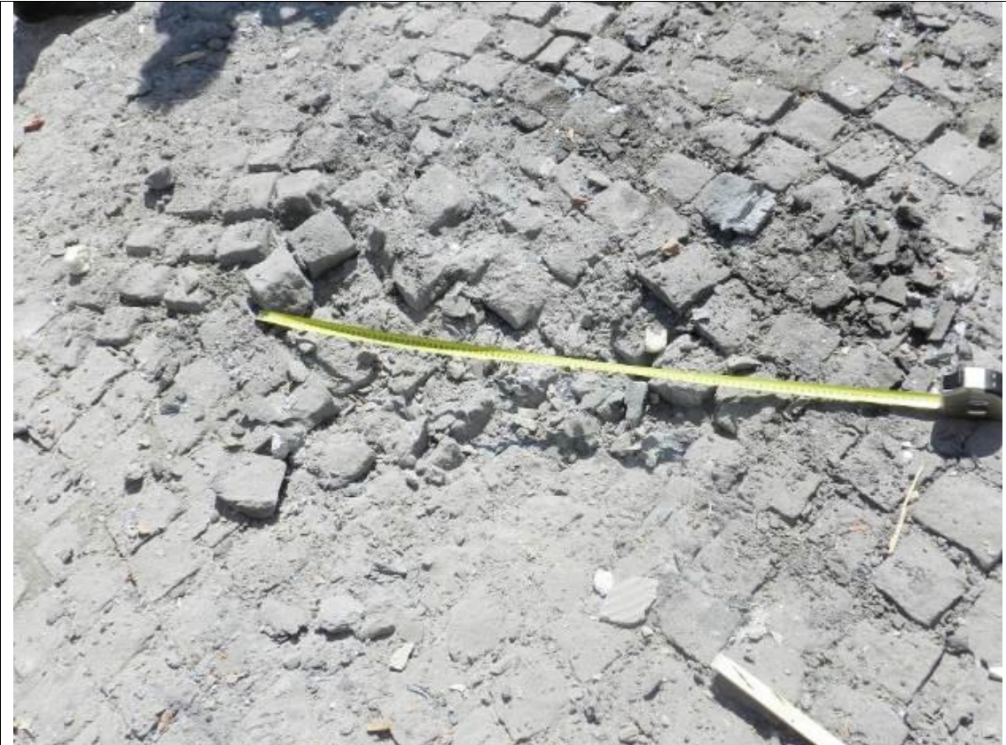
Figure 41 - The crater on the place of explosion at Testing Ground Nikinci, August 29, 2014.
