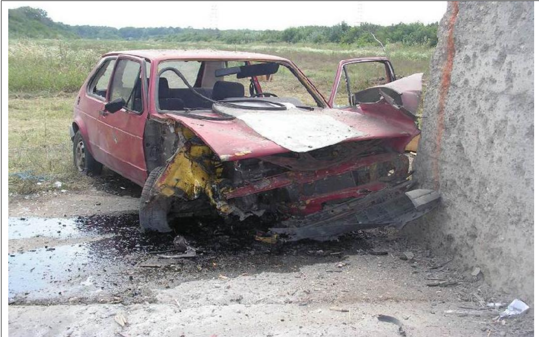
Figure 20 – The vehicle, type “Golf 1“ after the activation of 130 mm OF482M projectile placed under the 62° angle in relation to the horizon (photograph PICT0754)
