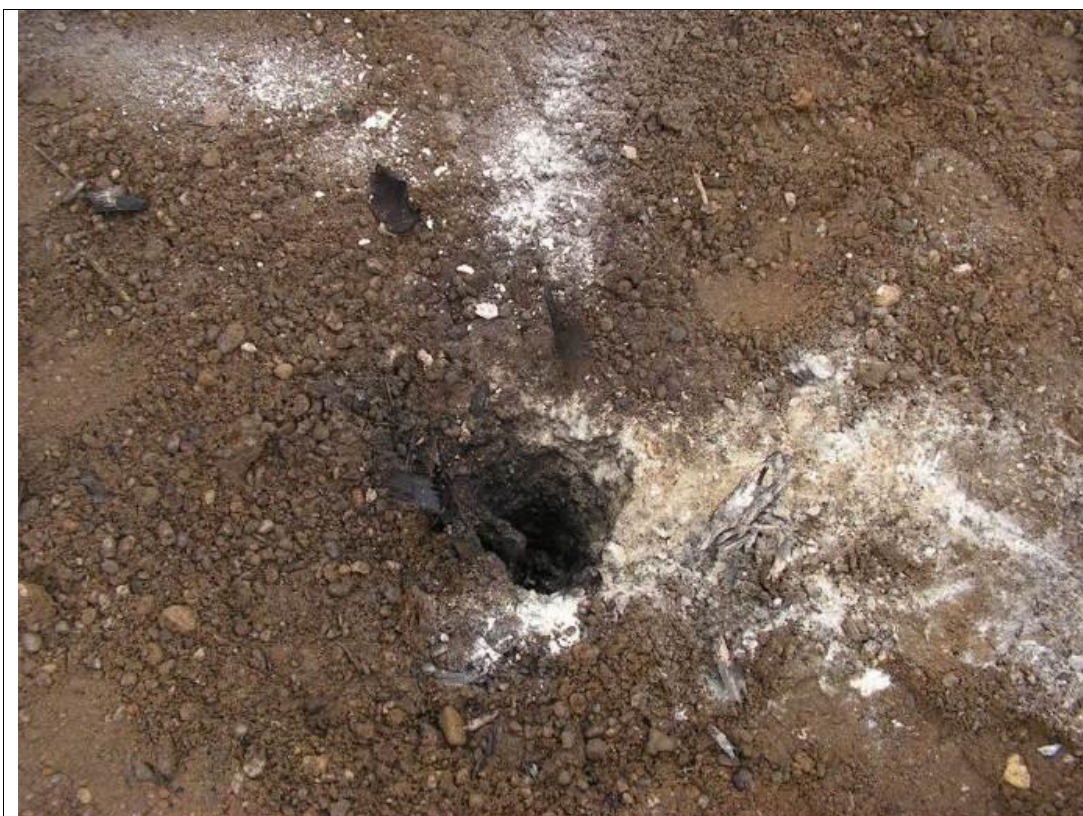
Figure 63 – The place of activation of 155 mm M107 projectile after deflagration. White marks were caused by disbursement of the explosive. ( photograph PICT0532 )
