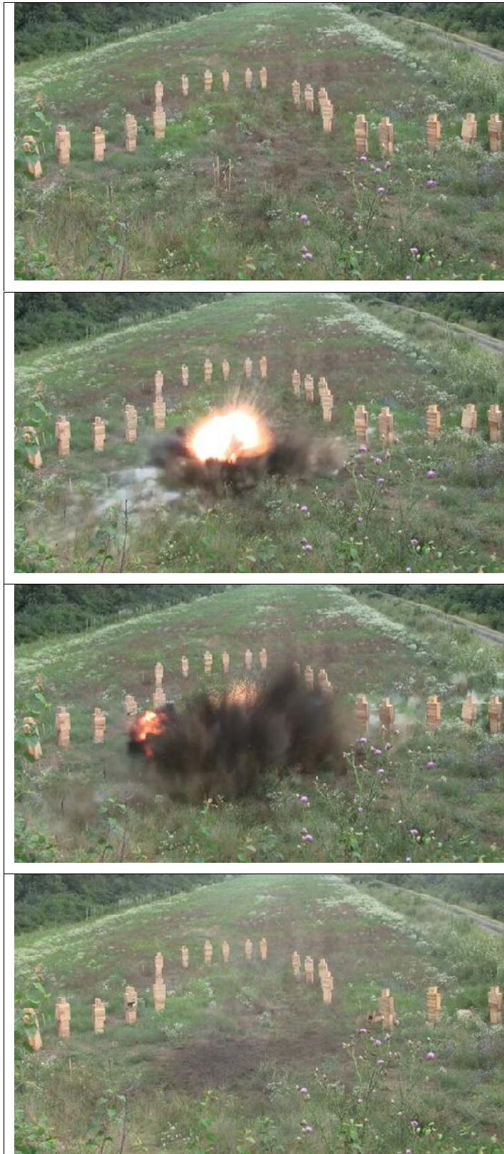
Figure 4 – The layout of the activation scene for the 130 mm M79 projectile, placed at the angle of 61^\circ to the horizon, before, during and after the explosion.
