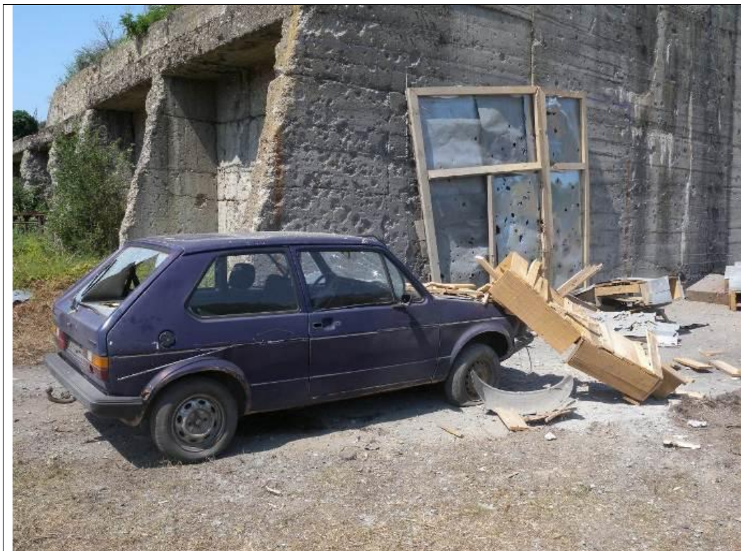
Figure 30 – The vehicle, type “Golf 1“ after the activation of 130 mm OF 482-M projectile placed at the 31° angle to the horizon ( photograph PICT0754 )
