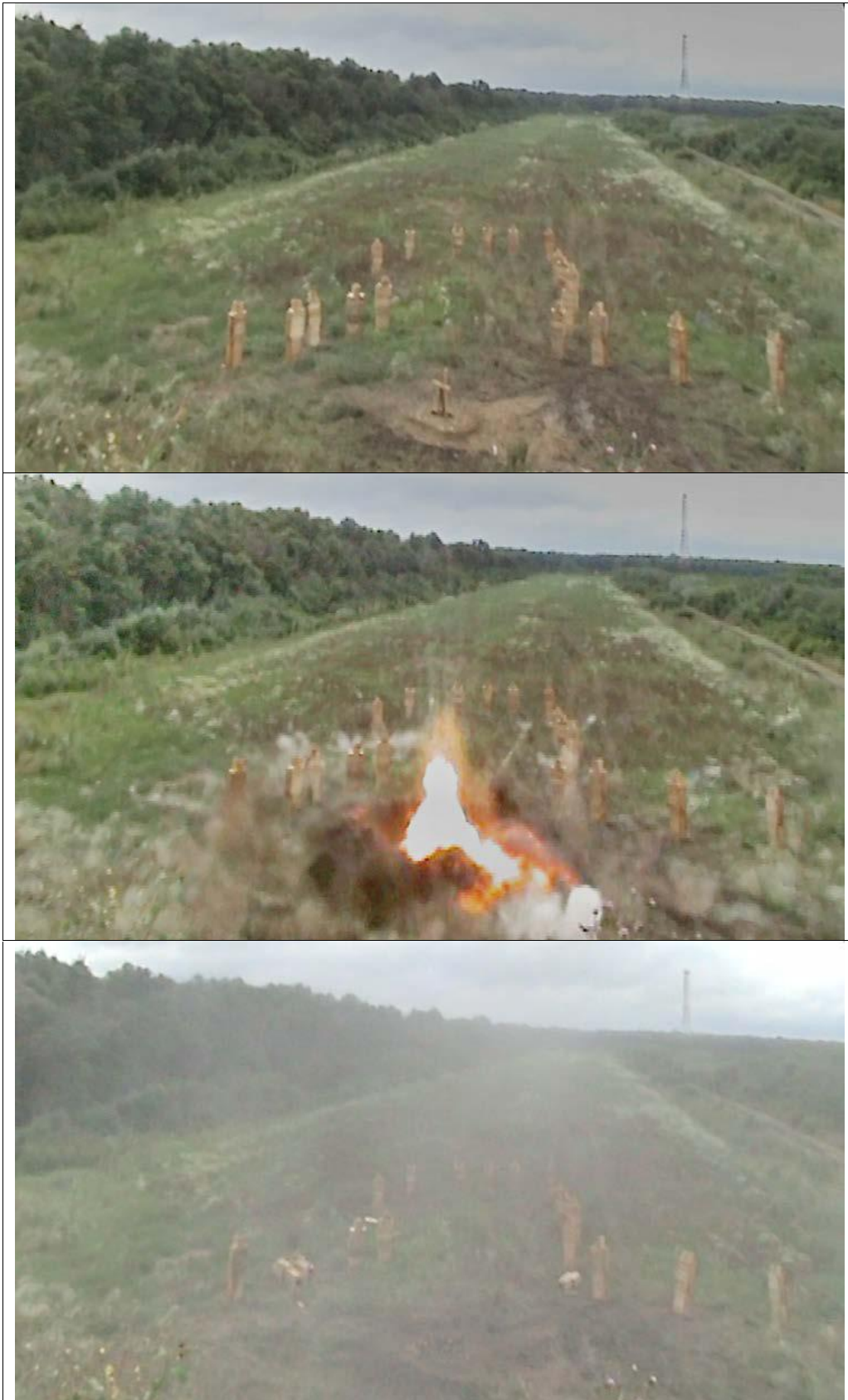
Figure 9 - The layout of human figure models, during the check of projectile spread for the 130 mm M79 projectile, at the angle of 90^\circ to the horizon, before and during the explosion.
