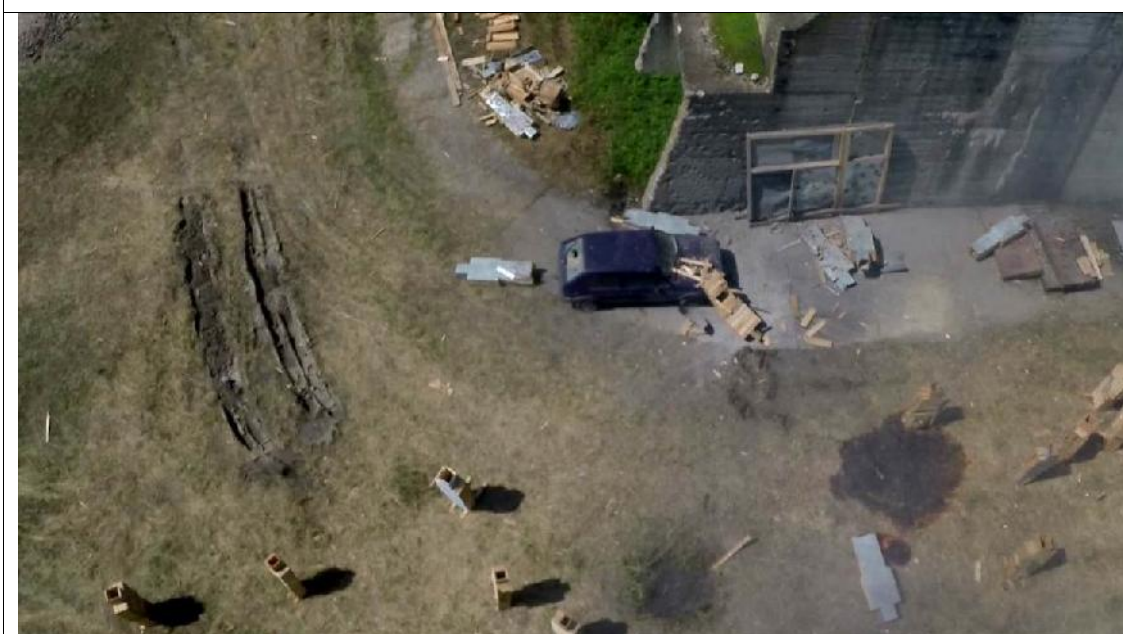
Figure 28a – The models and the car, before, during and after the explosion of 130 mm OF 482-M projectile at the 31° angle
