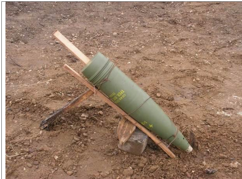
Figure 14 – Projectile 130 mm M79, placed at the 90° angle to the horizon
