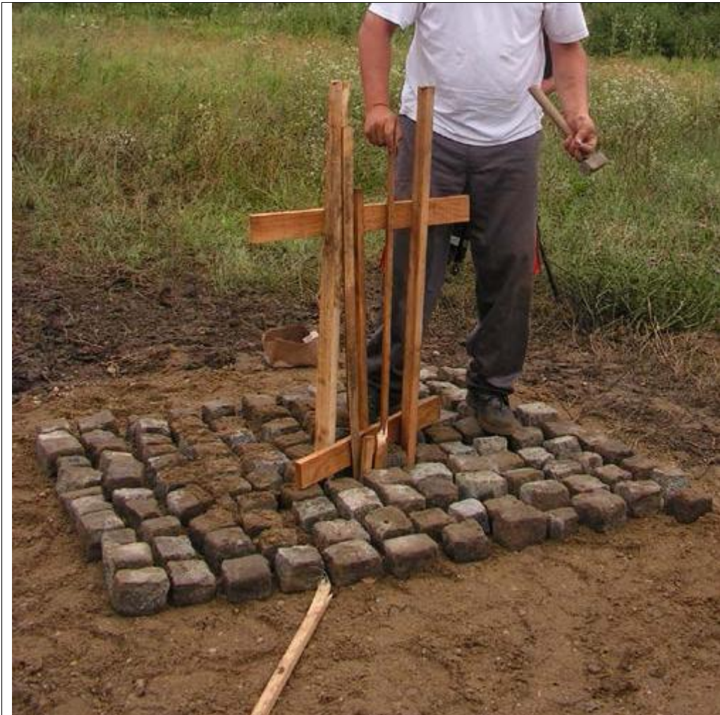
Figure 11 – The surface on which the 130 mm M79 projectile was activated at the 90° angle to the horizon
