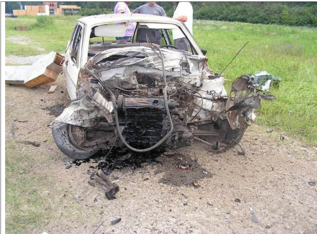
Figure 45 – The vehicle after explosion of 2,5 kg of PEP 500 explosive placed under the bumper (photograph PICT0125 )
