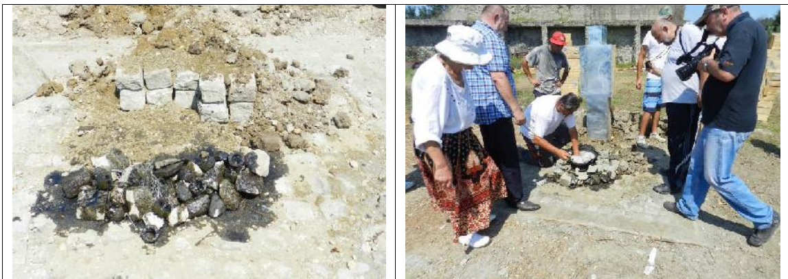
Figure 47 – The placement of 1 kg of PEP 500 plastic explosive on the granite cubes surface.
